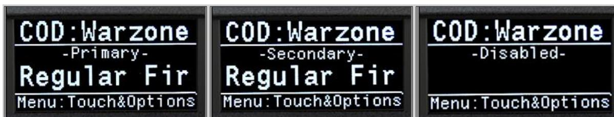
The Gearhead Eyes will display the active Weapon Profile as **Green for Primary**, **Red for Secondary**, or **Purple for Disabled**. If Weapon Swap (PS4 Solid Lightbar) is ON, the PS4 Lightbar will also display these colours.
